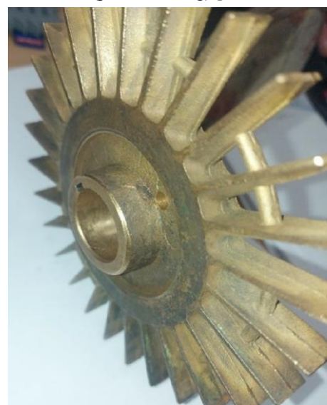
Fig. 2. Appearance of a shipboard pump impeller made using tin bronze casting technology [own materials].
