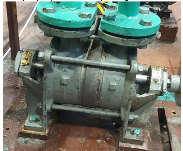
Fig. 1. SKA 5.01 hydrophore pump used in shipboard installations (part of test rig) [own materials].
