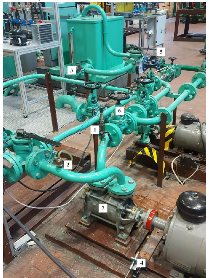
Fig. 5. Pump test bench (LESO) and diagram of the location of the sensors for the main operating parameters of the centrifugal pump. (1) discharge pressure sensor, (2) suction pressure sensor, (3) temperature measurement, (4) optical engine speed sensor, (5) flow meter with Hall sensor, (6) setpoint valve, (7) SKA 5.01 pump [own materials].
