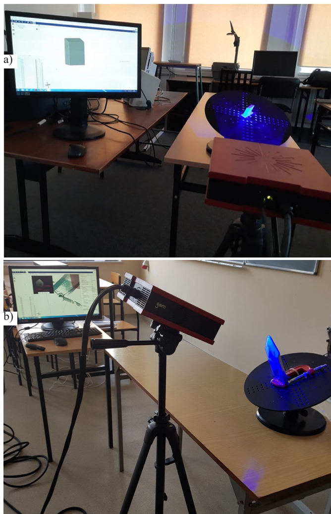
Fig. 8. The process of 3D scanning of: a) specimen; b) chisel
