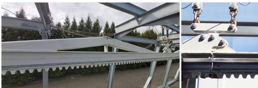
Fig. 1. View of the reinforced rail and double sling coupler built on a route intended for high-speeds [5]
