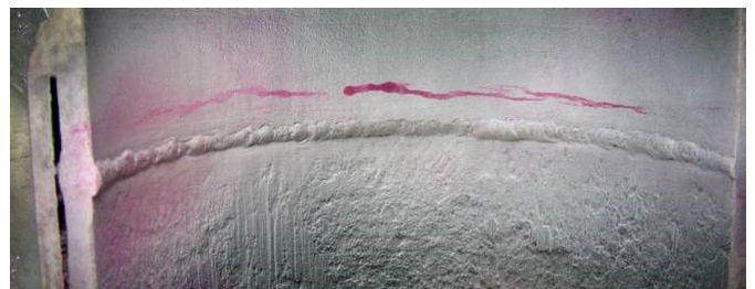
Fig. 9. View of the C1 welded joint from the inside of the pipeline after penetration testing
