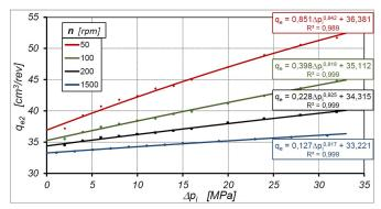
Fig. 12. Characteristics of  $q_{e2}$  vs  $\Delta p_i$  at n=const – according to Balawender's method
