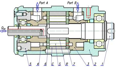
Fig. 4. Tested motor (satellite motor) [36, 37, 39]: C – curvature, S – satellite, R – rotor, 1 – shaft, 2 – case, 3 – inflow/outflow manifold, 4 – outflow/inflow manifold, 5 – rear body, 6 and 7 – distribution (compensation) plates
