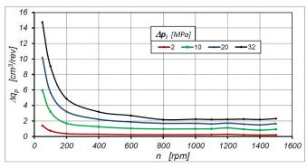
Fig. 15. Characteristics of  $\Delta q_p$  plotted according to equations from Table 1
