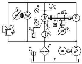
Fig. 6. The test stand measuring system [36, 37, 41]: P-pump, M-tested motor, PN-pump for filling leaks in P and M, IP-impeller pump, SV-safety valve, F-filter, T-tank, IAG-intersecting axis gear,  $E_1$  and  $E_2-electric$  motors with frequency converters,  $T_1$ ,  $T_T-temperature$  sensors,  $Q_2-flow$  meter,  $Q_{Le}-leak$  age measurement, FT-force transducer for torque measurement, n-inductive sensor for measure of rotational speed.
