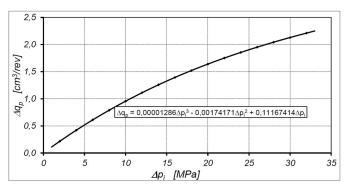
Fig. 16. Characteristics of  $\Delta q_p$  vs  $\Delta p_i$  for n > 800 rpm
