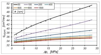
Fig. 13. Characteristics  $q_{e2(pH)}$  vs  $\Delta p_i$  at n = const - according to the new method. Equations in Table 1
