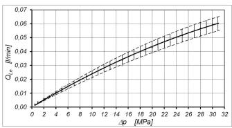
Fig. 9. External leakage  $Q_{Le}$  in tested motor [36]
