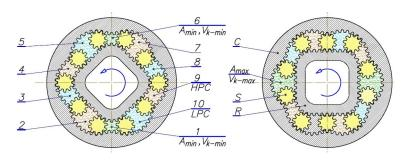
Fig. 5. Working (satellite) mechanism [23, 34, 36, 37, 41, 54]: C – curvature, R – rotor, S – satellite,  $1\div 10$  – working chambers, HPC – high pressure chambers, LPC – low pressure chambers,  $V_{k\text{-min}}$  – dead chamber,  $V_{k\text{-max}}$  – working chamber with maximum volume and with maximum area  $A_{\text{max}}$
